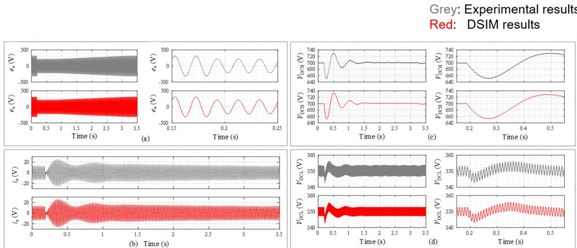
(a) grid-side voltage (b) grid-side current (c) high-voltage side DC-link voltage (d) low-voltage side DC-link voltage
