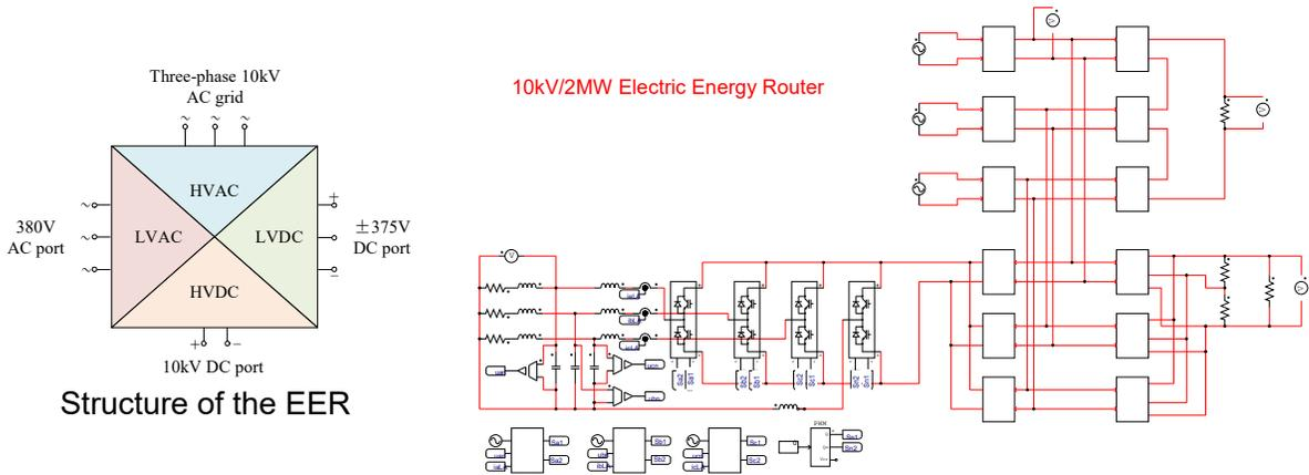
To simulate a 0.2s dynamic, DSIM takes only 17 seconds, which is more than 1000 times faster than a commercial software specialized in power electronics, while the simulated results are very close, with less than 0.01% relative error, as shown below. DSED represents the DSIM algorithm.
