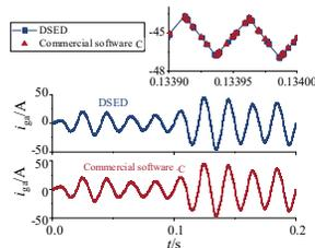
Simulated results comparisons of HVAC phase A grid-side current
