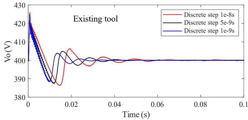
With 1e-9s time step, existing tool takes more than 20 minutes for 0.1 second simulation. However, with the Discrete State Event-Driven algorithm, DSIM takes less than 1 second to get the same results, which is more than 1300 times faster. The following figure shows the comparisons of the simulated results, where  $V_o$  is the output DC voltage, and  $V_{cr}$  is the resonant capacitor voltage. The tests are conducted with an Intel Core i7-6600U CPU.
