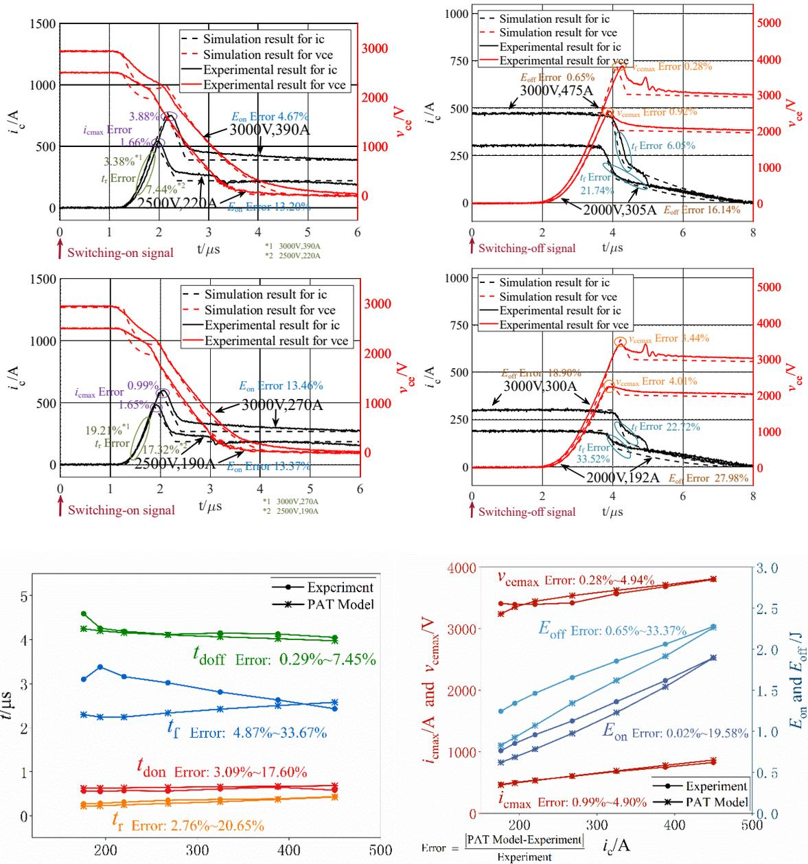
Generally PAT model gives good results compared with experimental waveforms, if the input parameters are accurate enough. Under some small-current conditions, the model error can be larger.
