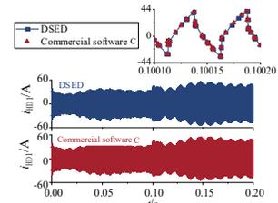
Simulated results comparisons of HVDC module 1 transformer current
