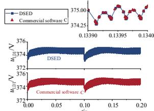
Simulated results comparisons of LVDC output voltage
