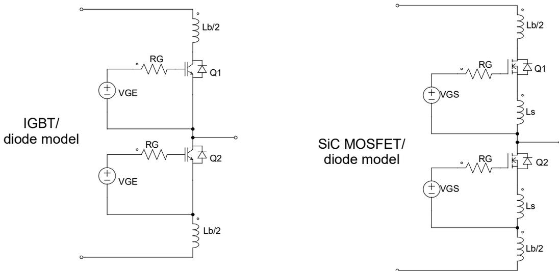
DSIM now offers transient model for all the switching modules except three-level NPC bridges. One can choose between IGBT/diode model and SiC MOSFET/diode model. Please turn to online help for more information about the definitions of the model parameters. In **Chapter 3 Examples**, comparisons of the model results and experimental results will be presented.
