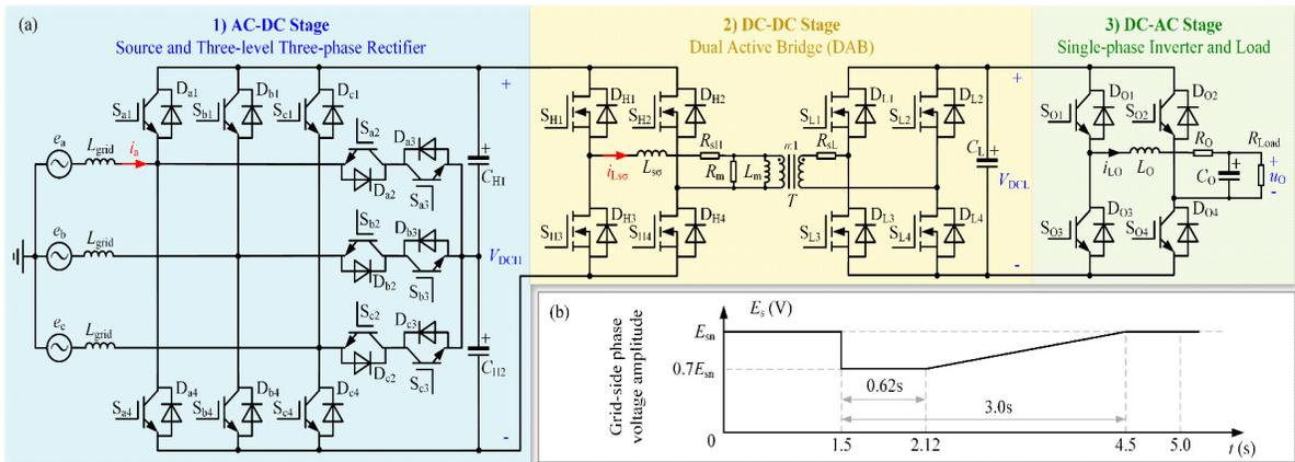
Overall circuit of the 50kVA SST and simulated low-voltage ride-through dynamic
