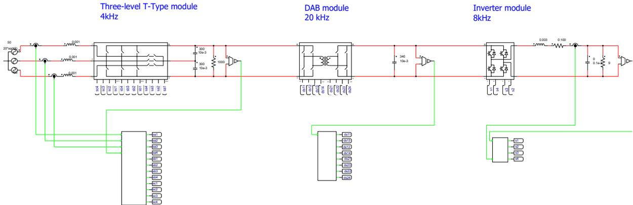
For the 5-second dynamic, if ideal switch model is used, DSIM takes less than 5 second to finish the simulation, which is about 50 times faster than current software; if transient switch model is used, DSIM takes about 50 seconds, which is 700 times faster than another commercial software. The comparisons are shown as below. The tests are conducted with an Intel Core i7-7700K CPU.
